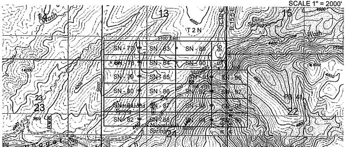
The above map depicts the SN 88 Lode mining claim, which is located in Section(s) 24 East. Gila and Salt River Baseline and Meridian, Gila County, Arizona. 2 North, Range 15 The claim corners, end centers and Location monuments are marked by 2 inch by 5 foot wooden post with aluminum tags. The bearings and distances between claims and tie point are depicted on the map.
