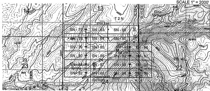
The above map depicts the SN 84 Lode mining claim, which is located in Section(s) 13 & 24. Township 2 North, Range \_\_\_\_15 \_\_\_ East. Gila and Salt River Baseline and Meridian, Gila County, Arizona. The claim corners, end centers and Location monuments are marked by 2 inch by 2 inch by 5 foot wooden post with aluminum tags. The bearings and distances between claims and tie point are depicted on the map.
