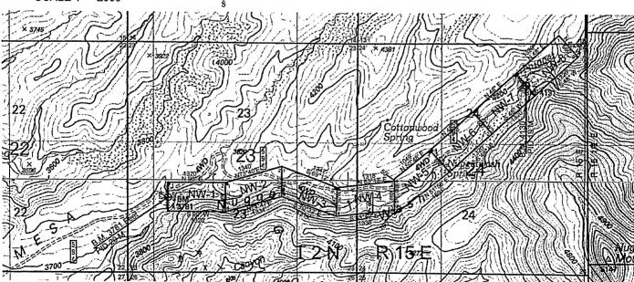
The above map depicts the placer mining claim, which is located in Section(s) 24 East, Gila and Salt River Baseline and Meridian, Gila County, Arizona. North, Range 15. The claim corners and Location monuments are marked by 2 inch by 5 foot wooden post with aluminum tags. The bearings and distances between claims are depicted on the map.
